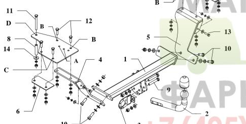
This towing hitch is designed to assembly in following cars: SUZUKI SX4, 2 WD and FIAT SEDICI, 2WD, both produced since 2006, catalogue number W25 and is prepared to tow trailers max total weight 1200 kg and max vertical load 50 kg.
